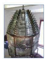
The light must be visible from afar. In 1821, the ingenious Fresnel lens was invented. It used glass prisms to collect & concentrate the light, allowing its detection from very great distances. It's been called "the invention that saved a million ships".
