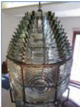
The light must be visible from afar. In 1821, the ingenious **Fresnel lens** was invented. It used glass prisms to collect & concentrate the light, allowing its detection from very great distances. It's been called "**the invention that saved a million ships**".
